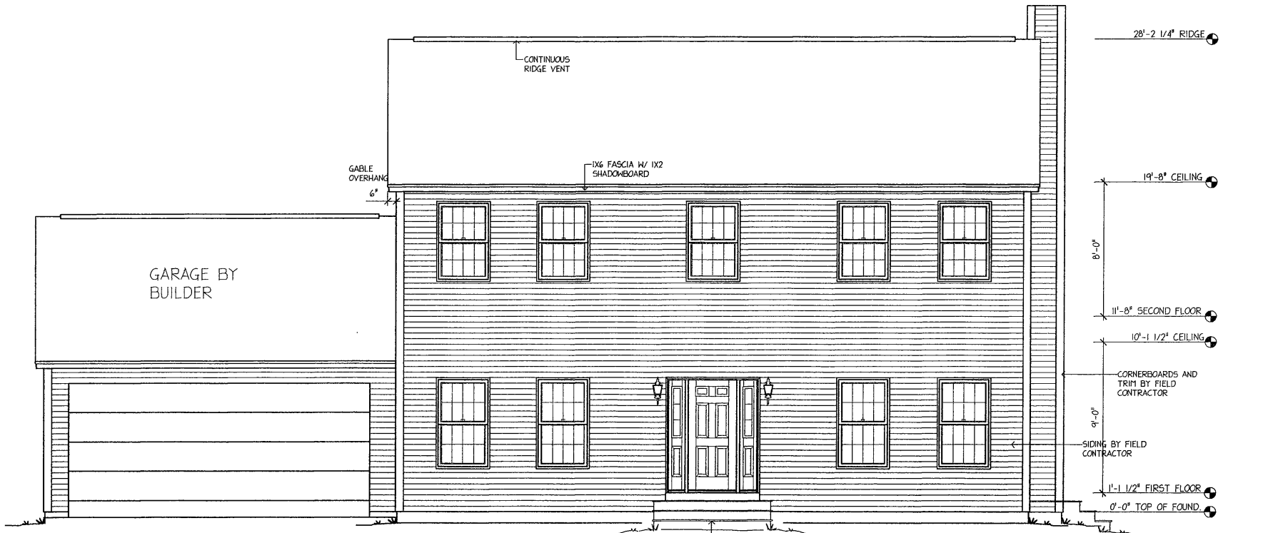
E-1 FRONT ELEVATION SCALE: 3/16" = 1'-0"
